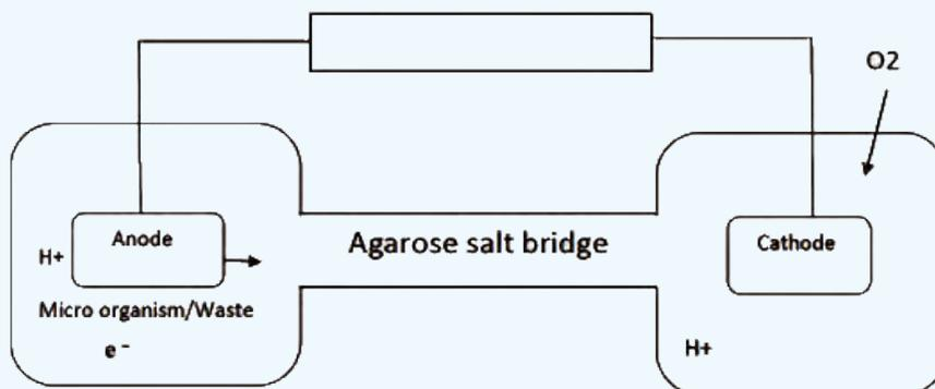
**Fig.1 Schematic diagram of double chambered MFC**
