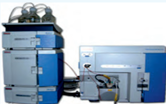
Liquid Chromatography Mass Spectrometer (LC MS MS) for molecular fragmentation and confirmation of Veterinary drugs
