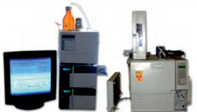
High performance Liquid Chromatography (HPLC) for identifying Mycotoxins
