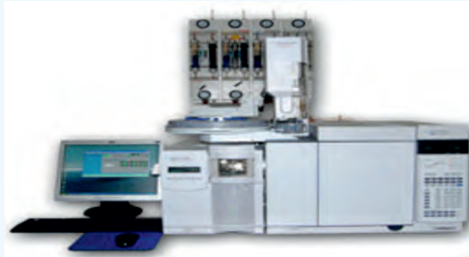
Gas Chromatography Mass Spectrometer (GC MS) for molecular fragmentation and confirmation of Melamine and Pesticides
