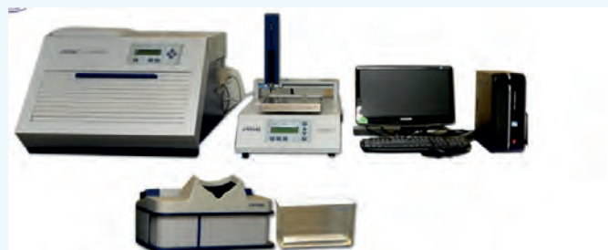
High Performance Thin Layer chromatography (HPTLC) for Screening of Mycotoxins, Pesticides and Veterinary Drugs
