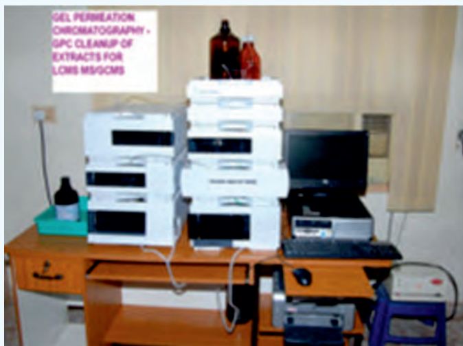
Automated Gel Permeation Chromatography (GPC) for cleanup of samples prior to LC MS MS/GC MS identification
