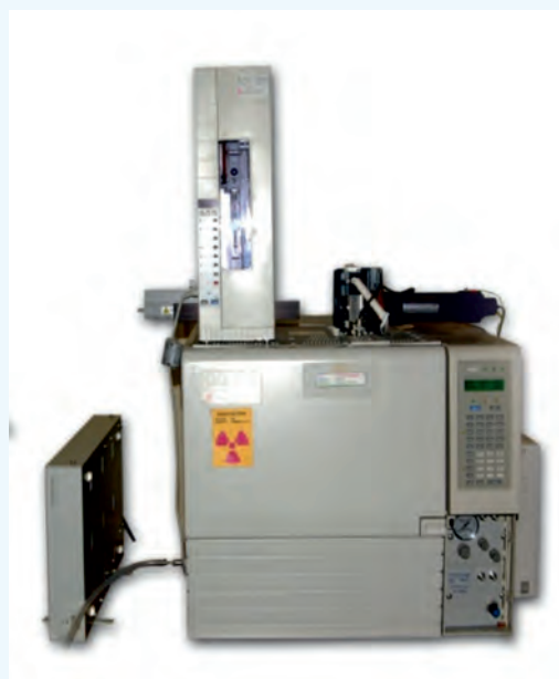
Gas Chromatography (GC) for identifying Pesticides
